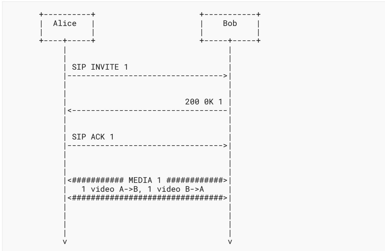
In SIP INVITE 1, Alice sends Bob a SIP INVITE including the basic audio and video capabilities and data channel in the SDP body as per [RFC8841](#). Alice also includes the "sip.clue" media feature tag in the INVITE. A snippet of the SDP showing the grouping attribute and the video
