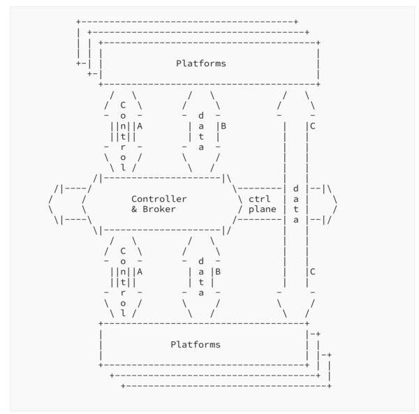
Figure 1: XMPP-Grid Architecture
