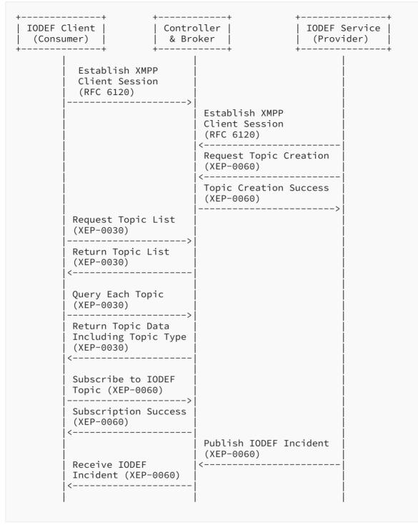
Figure 2: IODEF Example Workflow
