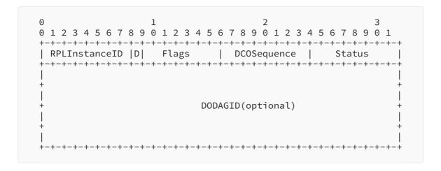
Figure 4: DCO-ACK base object
